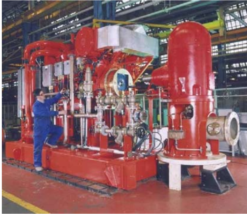
FIGURE 9 Zeron 100 firewater pump for the South Arne project.
