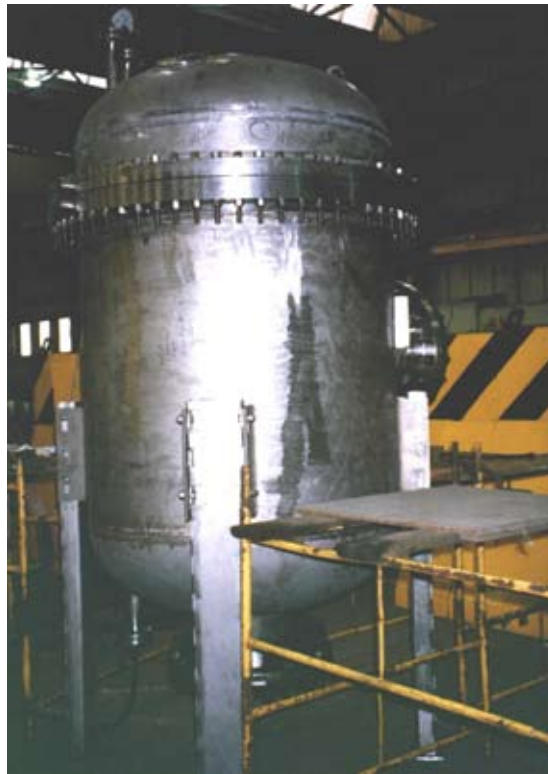
FIGURE 13 Seawater filter vessel in Zeron 100 for the BP Bruce project.
