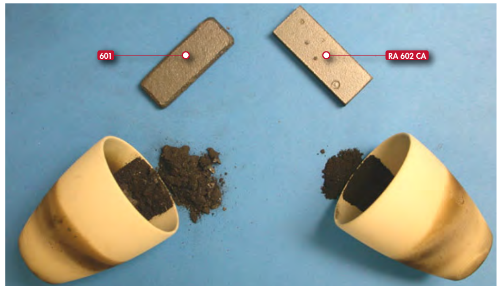
RA 602 CA vs alloy 601 after 3026 hours at 2250°F.
