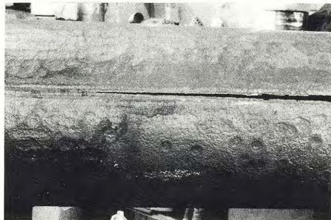
Fig. 14 Oxidized weld in rotary retort 1/4 X
