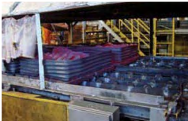
Fig. 4. RA 253 MA corrugated boxes shown cooling down upon exiting an isothermal annealing operation at 1750°F.
