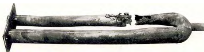
Fig. 3: Broken radiant tube
