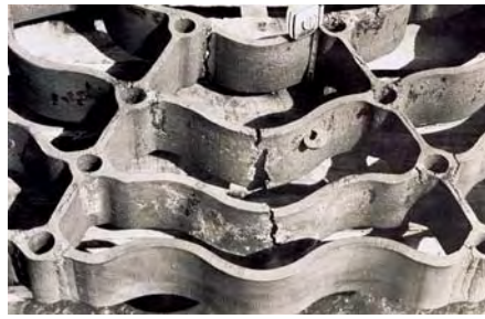
Fig. 7: Effect of cast alloy surface and internal defects versus wrought alloy soundness
