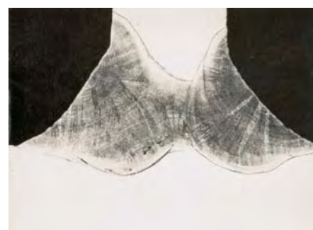
Fig. 6a: This fully welded joint can resist both thermal and mechanical fatigue
