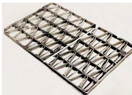
Fig. 5: Serpentine tray of 6 and 9.5 mm RA 330
