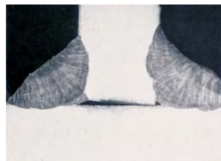
Fig. 6b: The unfused void in this fillet weld acts as a stress riser and may cause premature failure
