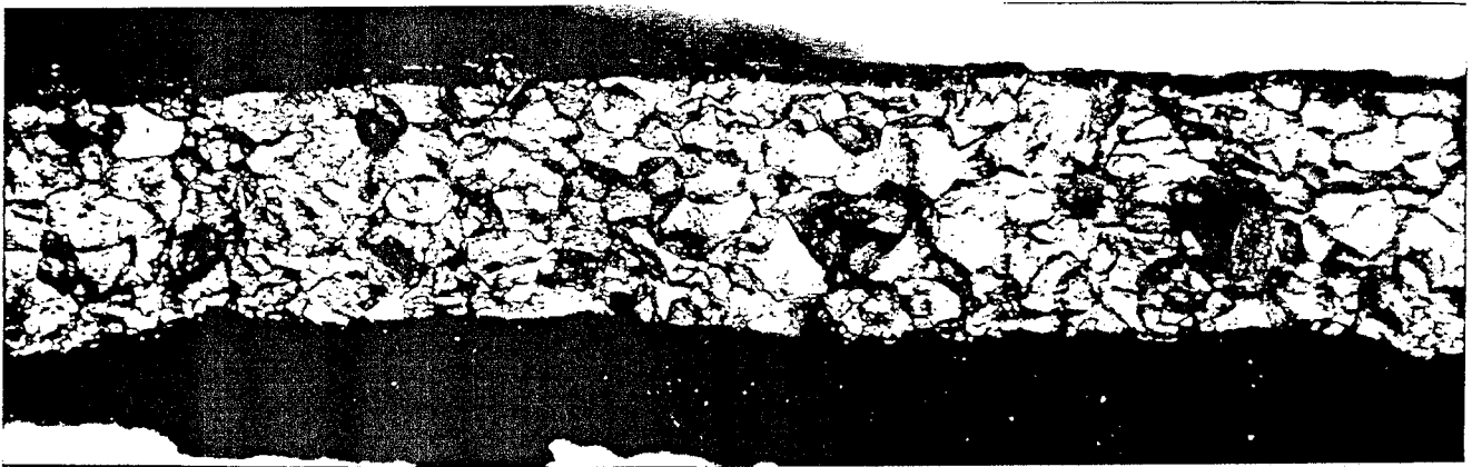
Figure 2A: Brittle fracture of an alloy 601 corrugated muffle from the combination of extensive grain growth and carburization
